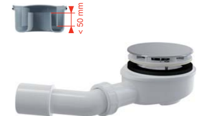
A492CR Shower waste and trap for thick-walled trays, reduced height, waste outlet 90 mm, DN 50, plastic, chrome-polished
