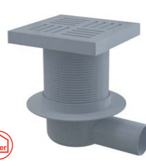
APV5211 Floor drain 150×150/50 mm side outlet, grey grid, wet odour trap
