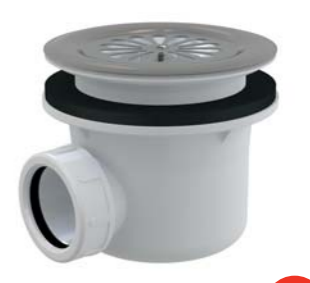
A48 Shower waste and trap, waste outlet 90 mm, DN 40, grid Ø 115 mm, metal, stainless steel-polished
