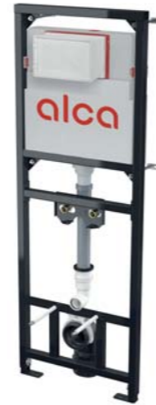
A108F/1500 Mounting frame with cistern for a waste sink with waste connection DN90/110 and faucet
