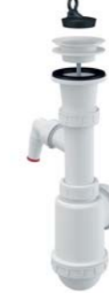
A442P-DN50/40 Sink waste and trap DN 40/50 with Ø 17-23 mm connector and plastic grid Ø 70 mm, rubber plug
