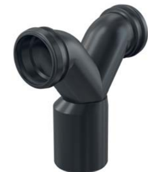
M909 Double elbow waste connector 90° for wall-hung WC, reducer 2x DN 90 x DN 110, length 253 mm, PE, black
