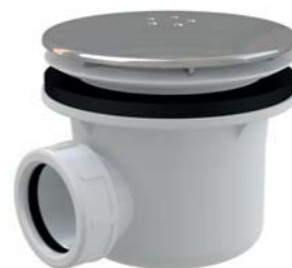
A49K Shower waste and trap, waste outlet 90 mm, DN 40, metal, chrome-polished
