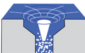
Normal roof drain
